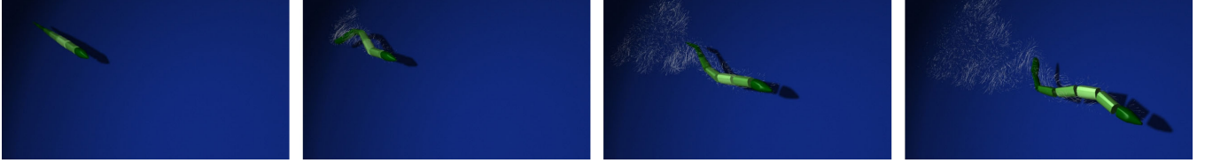
Figure 7: A swimming seven-link eel. Anguilliform swimmers undulate their whole body as if a wave is travelling from head to tail, and shed two separate trails of vortices from the tail.
